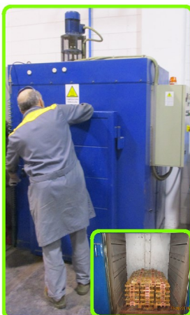
SHUNT 4000A - HEAT TREATMENT OVEN
